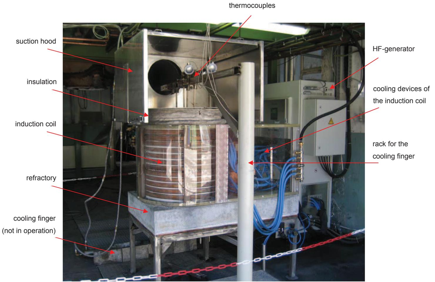
figure 6: testing facility
